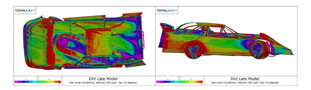
CFD provides aero data, allowing for the exploration and optimization of a vehicle's performance under different scenarios. It offers the flexibility to enhance existing designs, making it a valuable tool for both elite teams and enthusiasts.
