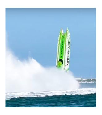
During the 2019 Race World Offshore World Championships, two Doug Wright 32' catamarans experienced a simultaneous "blow-over" incident in the Super Stock class race. The side-by-side configuration created compressed tunnel air, increasing pressure and causing the boats to flip. CFD analysis by TotalSim revealed the disruption in lift and downforce balance, leading to instability.
